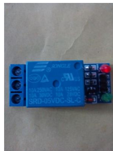
Figura 3 Relé o Relay
