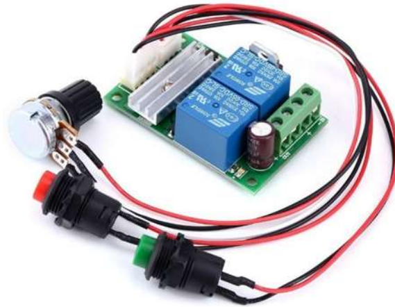
Figura 8: Control motor DC, inversor de giro, 24V/3A
