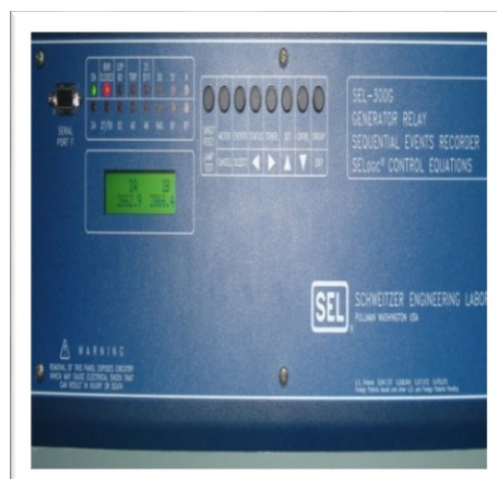
Figura 41. Relé SEL-300G. Panel frontal
