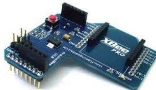
Figura 6.5: Xbee Shield
