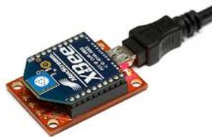
Figura 6.4: Xbee Explorer USB
