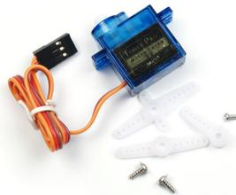
Figura 6.1: Servo SG90 - Tower Pro
